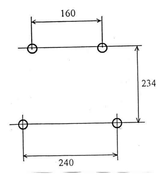
Hole axis spacing needed for the installation.
